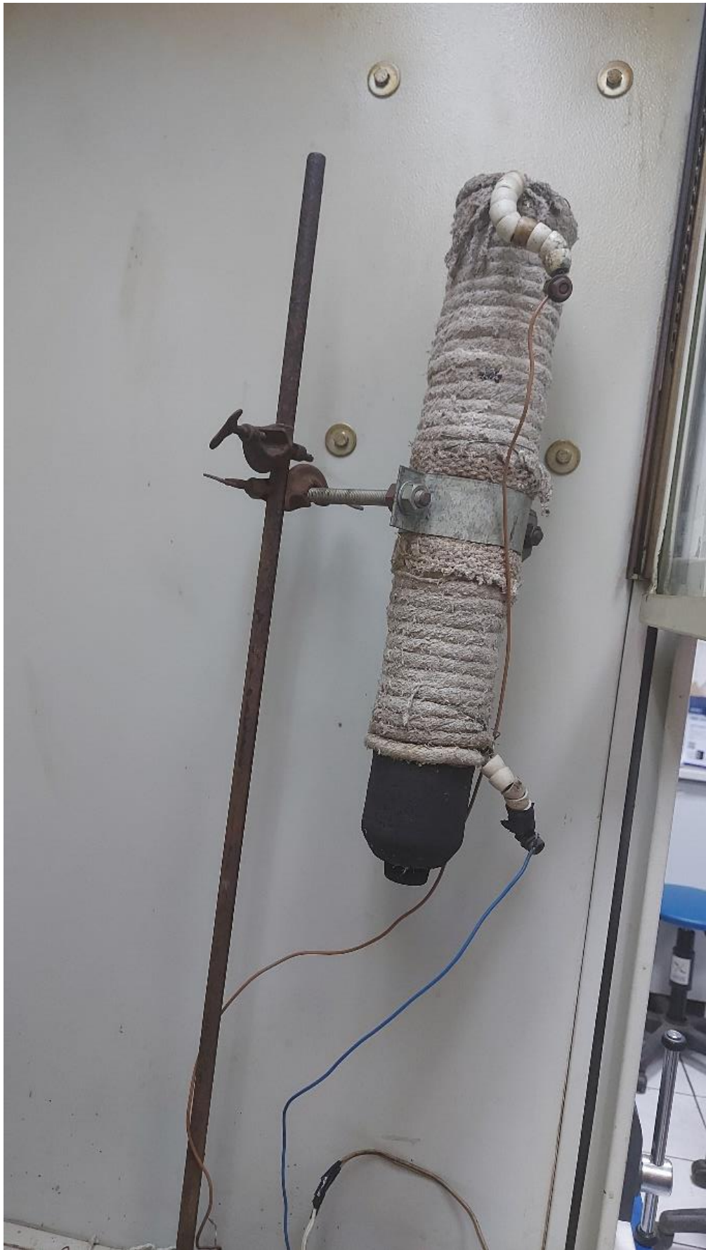
Figure 2 - Installation for superheated steam activation
