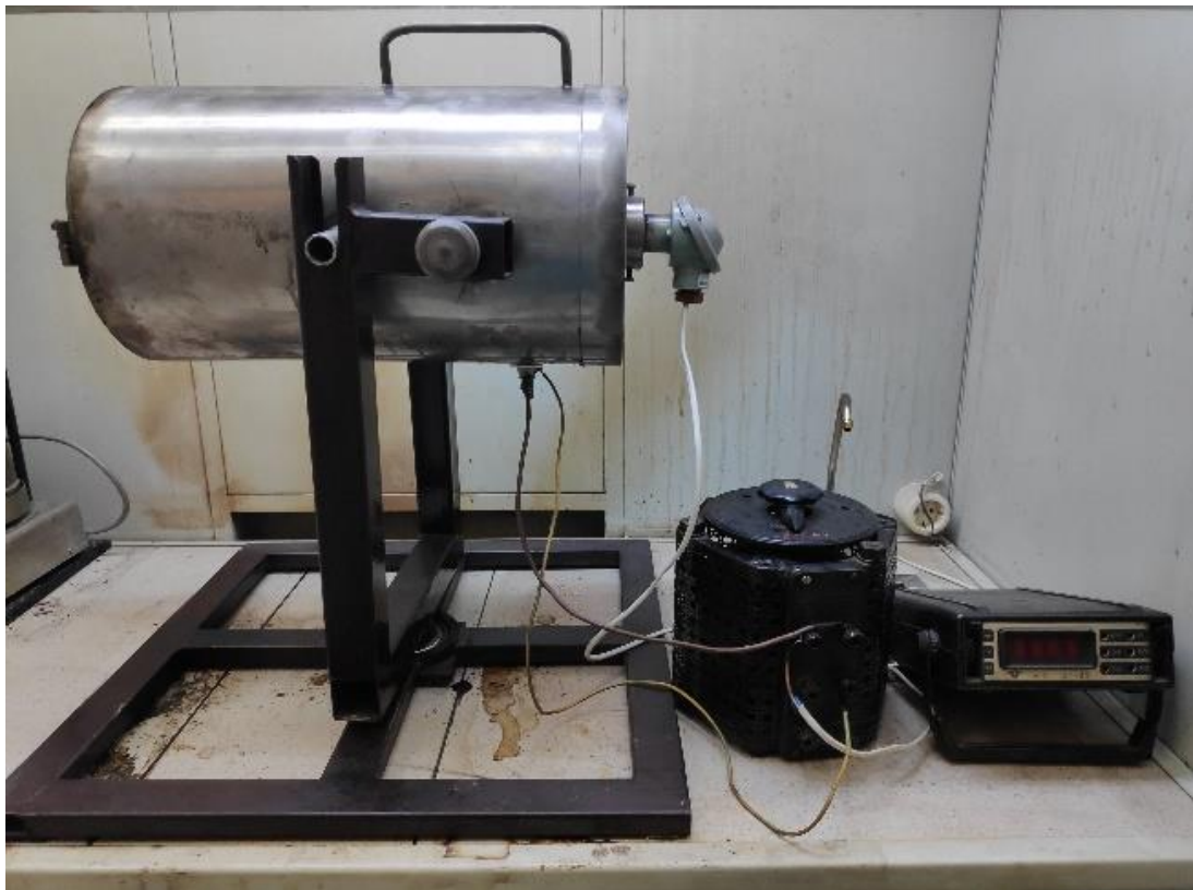
Figure 1 – Installation for the Carbonization of Vegetable Raw Materials in an Inert Atmosphere
